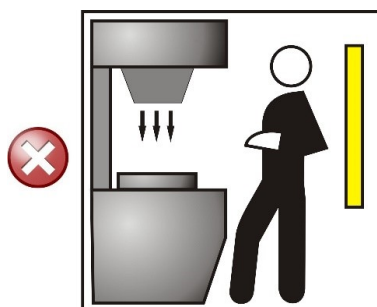
Figure 8: Wrong light curtain positioning
