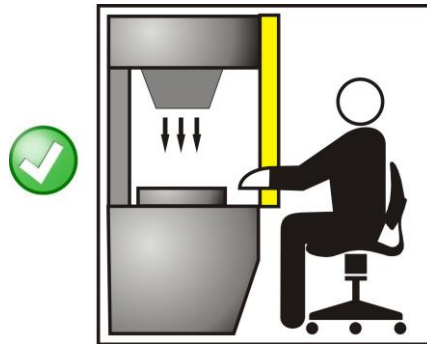
Fig 8 - Correct light curtain positioning
