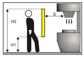
Fig 3 - Installation distance (vertical positioning)
