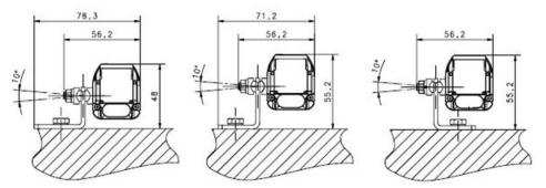
Fig 46 - Angled fixing bracket + Orientable support
