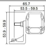
Fig 50 - Angled fixing bracket
