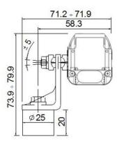
Fig 53 - Angled fixing bracket + Orientable support + Antivibration support
