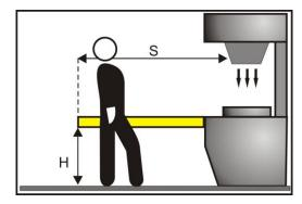
Fig 4 - Installation distance (horizontal positioning)
