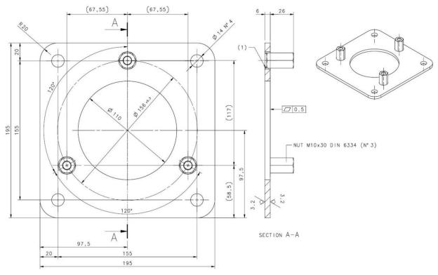
Fig 57 - Dimensions (mm)
