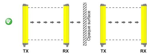
Fig 17 - Recommended positioning for homologous devices
