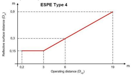
Fig 14 - Minimum distance from reflective surface
