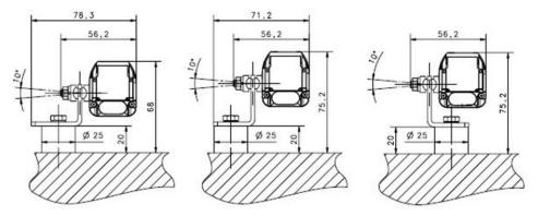
Fig 48 - Angled fixing bracket + Orientable support + Antivibration support
