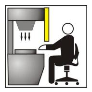
Fig 9 - Wrong light curtain positioning
