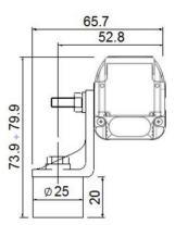
Fig 52 - Angled fixing bracket + Antivibration support
