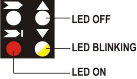
Fig 41 - Signalling LEDs
