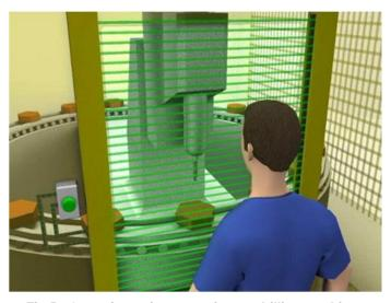
Fig 5 - Operating point protection on drilling machines
