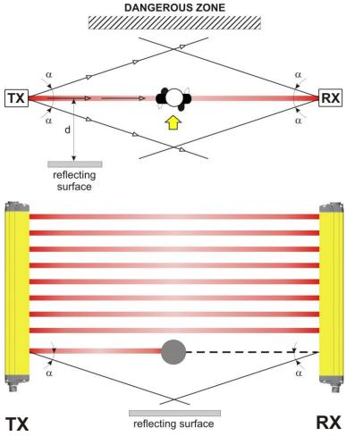
Fig 13 - Distance from reflecting surfaces
