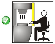
Fig 10 - Correct light curtain positioning
