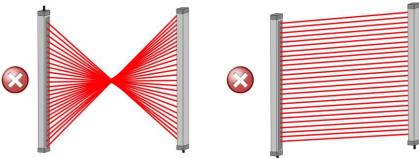
Fig 18 - Wrong light curtain TX-RX orientations
