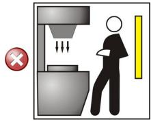
Fig 11 - Wrong light curtain positioning
