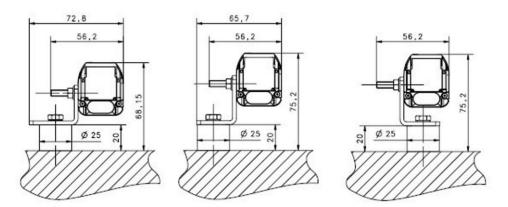
Fig 47 - Angled fixing bracket + Antivibration support
