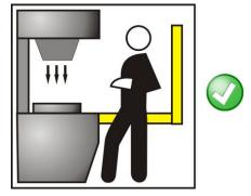
Fig 12 - Correct light curtain positioning
