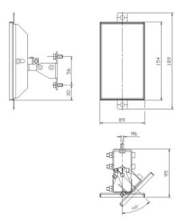
Fig 61 - SG-DM 150 Dimensions (mm)
