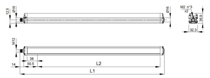
Fig 42 - Dimensions (mm)
