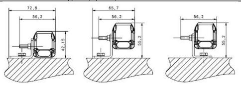
Fig 45 - Angled fixing bracket
