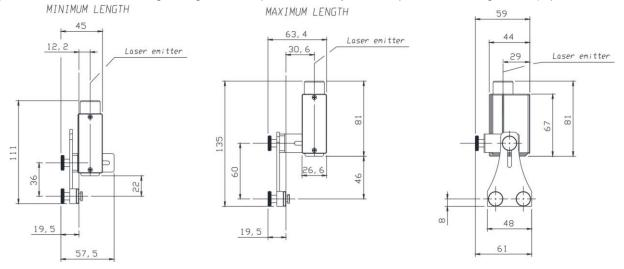
Fig 68 - Dimensions (mm)
