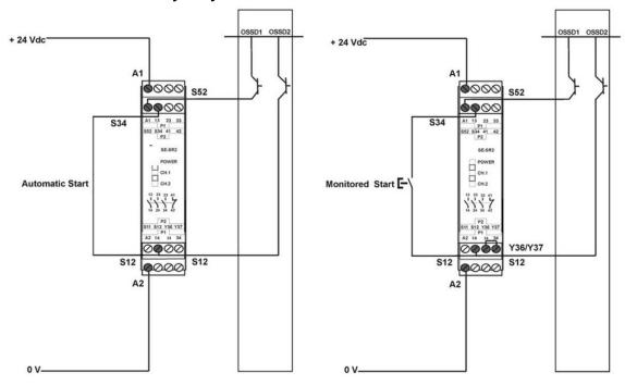
Fig 29 - Connection to SE-SR2 Safety Relais
