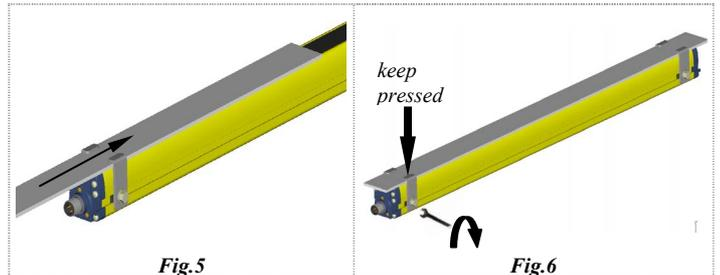
**NOTE:** ESPE maximum operating distance is reduced of 10% for each couple of "LENS" SHIELD" used (one for TX unit and one RX unit).
