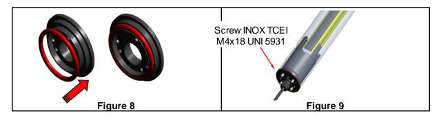
Finally, tighten the 4 INOX TCEI M4x18 UNI 5931 screws (max. tightening torque 0.8 Nm) on both sides for the complete compression of the O-ring seal against the tubular inner surface (Fig.9).
