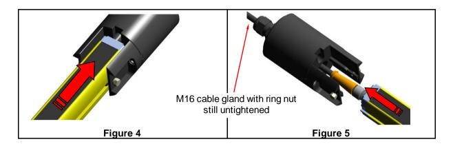
When both part  $\mathbf{b}$  and  $\mathbf{c}$  are completely installed, firmly tighten the gland nut to fix the cable. Check once again that the M5x6 UNI TE 5739 screws are well tightened on their elastic washers.
