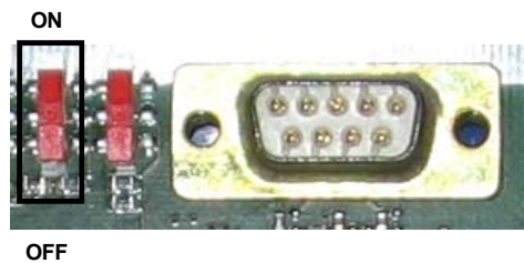
Figure 11 – RS485 HD Termination Resistance Switch
