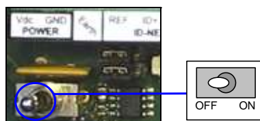
Figure 4 - Power Switch ON/OFF Positions
