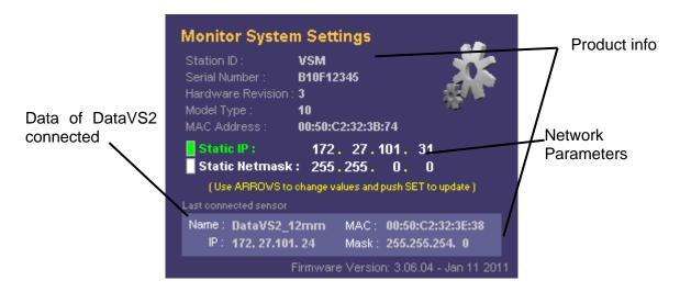
To change the network parameters, the user has to simply move the focus on the desired value and use the **UP/DOWN ARROWS** to increase or decrease the current value. To save the changes press **SET**.
