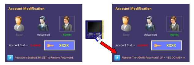
At this point the system requests the user to confirm the cancellation of the password. To confirm press **ARROW UP.**
