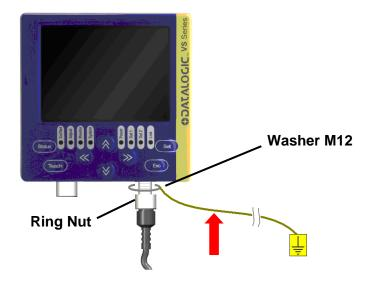
Insert the washer M12 on the yellow/green cable in the VSM connector and then screw the Ethernet cable until the ring nut reaches the washer.
