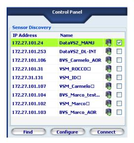
The control panel will display a list of all the DataVS2/VSMs found by the "Find sensor" function. The following information will be shown for each device:
