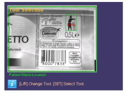
The "*Tool Selection*" panel is displayed and the user can choose the tools to use. All the inspection tools will be displayed one at time according to the creation order.
