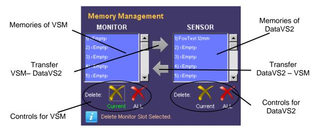
As shown in the figure, the panel is divided in two: a VSM area (concerning the local memory) and a DataVS2 area (remote device memory).
