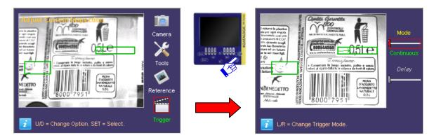
Parameters that can be modified are "Trigger Mode" and "Trigger Delay".
