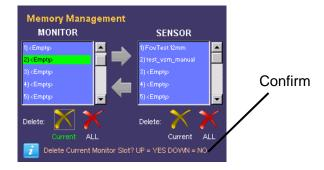
To proceed press **ARROW UP** otherwise, press **ARROW DOWN** to abandon. In both cases, the information label will display the operation result and a refresh of the panel names will be made.
