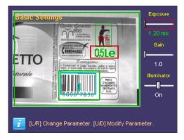
The user can change the focus between the objects on the panel by using the **UP/DOWN ARROWS**. To change the parameter value, once selected the focus, the user has to use the **RIGHT/LEFT ARROWS**.
