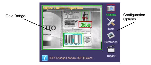
As you can see in the image, the VSM is split into two main areas: the field range of the camera and the configuration options available.
