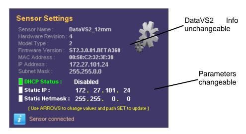
To change the network parameters of DataVS2, the user has to simply move the focus on the desired value and use the **UP/DOWN ARROWS** to increase or decrease the current value.
