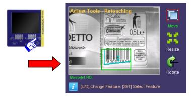
All the parameter change panels can be accessed from here on starting from the ROI panel up to the last one with the parameters that can be changed using the selected tool.
