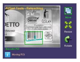
Once selected "Move", the focus is transferred in the field range and the ROI can be moved using the ARROWS. Once you have achieved the desired position, press **TEACH** to save changes. Press **ESC** to return to the Setup menu ignoring the changes made.
