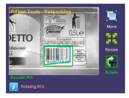
To rotate the ROI, select the "Rotate" option from the Setup menu (using the SET button again). The ROI will rotate in a clockwise/anticlockwise directly depending of the RIGHT/LEFT ARROW button pressed.
