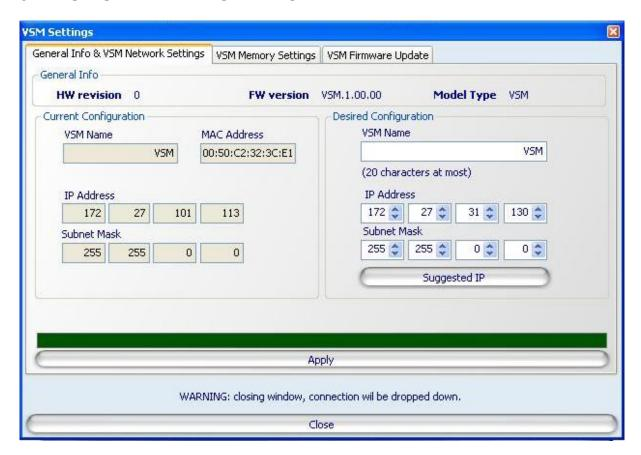
This window displays general information on VSM to which you are connected. Of the parameters displayed, you can change:
