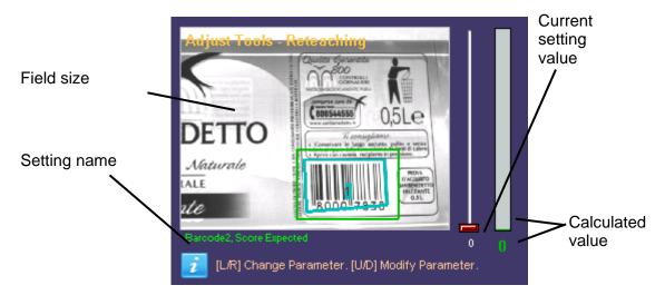
The parameters are displayed one at a time, and so the **RIGHT/LEFT ARROWS** must be used to pass from parameter to the another.
