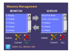
Another confirmation will be requested. To proceed press **ARROW UP** otherwise, press **ARROW DOWN** to abandon. In both cases, the information label will display the operation result and a refresh of the panel names will be made.
