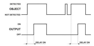
Select "dLOn" in the parameter menu to set the DELAY ON function.
