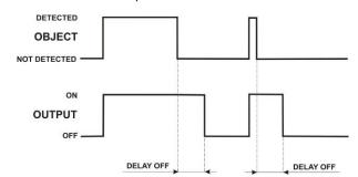
Select "dLOF" from the parameter menu to set DELAY OFF function. The parameter programming is accessed by pressing (SET). The previously set delay value appears on the display.
