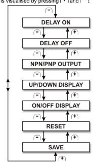
The DELAY ON represents the output delay activation after the reference mark has entered in the detection area. The delay avoids the detection of events that occur rapidly. An example can be a mark with shaded colours (light-dark-light) that can be detected twice
