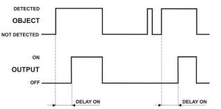
Select "dLOn" in the parameter menu to set the DELAY ON function. The parameter programming is accessed by pressing (SET). The previously set delay value appears on the display
