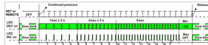
To choose the variation mode between increment or decrement of the OFFSET value, press SET or activate REMOTE twice rapidly (double click), in this way the sensor toggles between the two modes at each double click.
