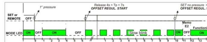
The OFFSET manual regulation mode is executed by pressing SET or activating REMOTE. The sensor will do the first five variations at the speed of 1/sec, the second five variations at the speed of 2/sec and the next variations at the speed of 5/sec, up to the SET or REMOTE deactivation or up to the reaching of minimum or maximum OFFSET value.
