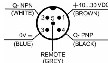
When the REMOTE wire is connected to 0V, it is as if the SET push-button was pressed.
