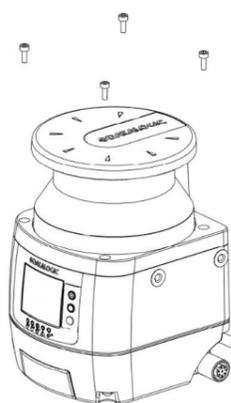
3. Remove the optical window with a linear, vertical movement.
