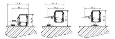
Figure 2 - Angled fixing bracket
