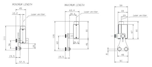
Figure 27 - Dimensions (mm)
