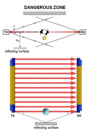
Figure 5 - Distances from reflective surfaces
