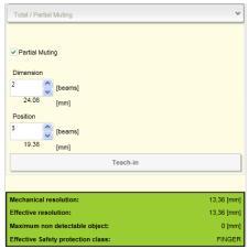
Choose correct parameters for selected zone. Both Dimension and Position are set in beams unit, equivalent measures in mm are exposed by GUI.
