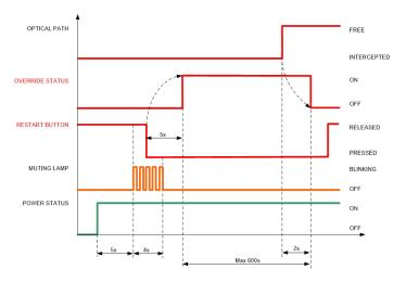
Figure 45 - Startup Override activation and timings
