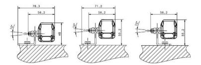
Figure 3 - Angled fixing bracket + Orientable support
