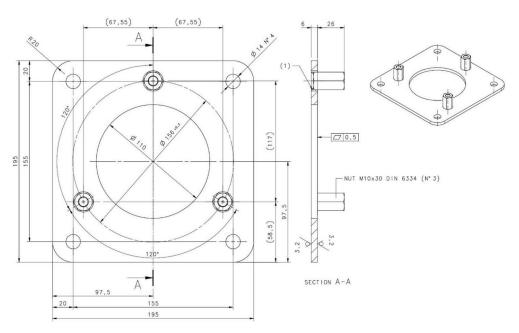
Figure 14 - Dimensions (mm)
