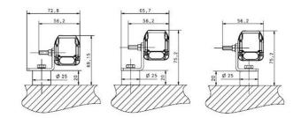
Figure 4 - Angled fixing bracket + Anti-vibration support
