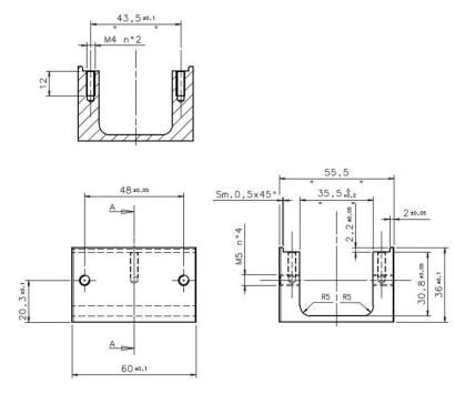
Figure 39 - Mounting bracket
