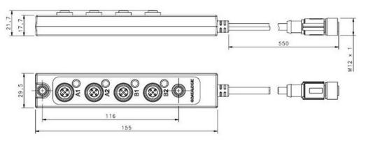
Figure 47 - Dimensions (mm)
