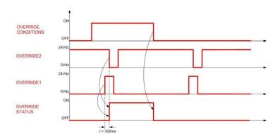
Figure 35 - Override timings (edge trigger)
