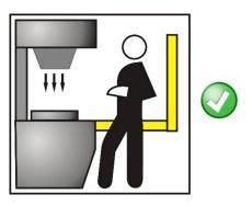
Figure 4 - Correct light curtain positioning
