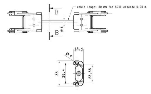
Figure 26 - CS-F1-80-B-0005 Dimensions (mm)
