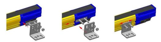
Figure 1 - Fixed brackets mounting procedure
