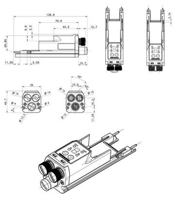
Figure 29 - Dimensions (mm)
