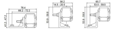
Figure 7 - Angled fixing bracket
