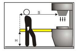
Figure 4 - Installation distance (horizontal positioning)
