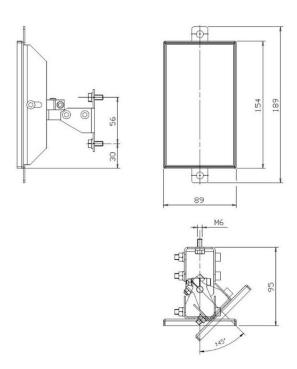
Figure 18 - SG-DM 150 (mm)
