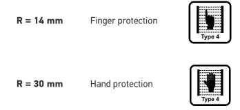
As shown in Figure 1 the resolution only depends on the geometrical characteristics of the lenses, diameter and distance between centers, and is independent of any environmental and operating conditions of the safety light curtain.
