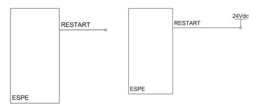
**Manual Restart:** after the ESPE has detected an opaque object in the controlled area, the light curtain begins its normal functioning only by pressing the Restart button (normal open push button) and after the object has been removed from the controlled area.
