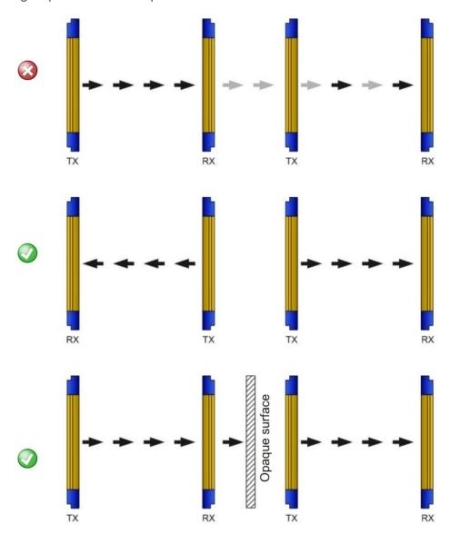
Figure 9 - Recommended positioning for homologous devices
