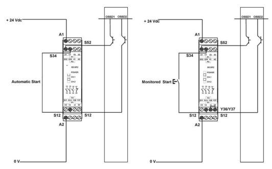
Figure 6 - Connection to SE-SR2 Safety Relays
