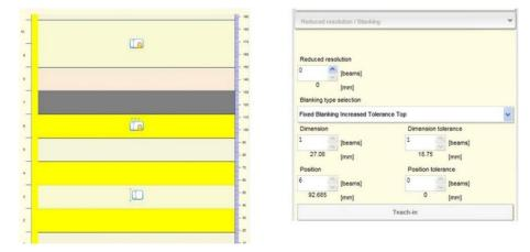
Figure 59 - Fixed Blanking with increase tolerance
