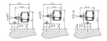
Figure 5 - Angled fixing bracket + Orientable support + Anti-vibration support
