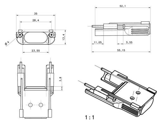
Figure 2 - Dimensions (mm)
