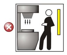
Figure 3 - Wrong light curtain positioning
