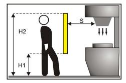
Figure 3 - Installation distance (vertical positioning)
