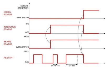
Figure 2 - SG4-P Restart timings (manual)
