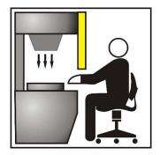
Figure 1 - Wrong light curtain positioning
