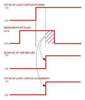
In Alignment Mode ESPE is always in Safe State and the OSSDs are kept OFF.
