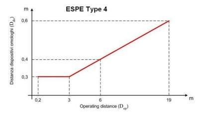
Figure 6 - Minimum distance from reflective surface
