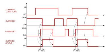
Figure 34 - Override timings (level trigger)
