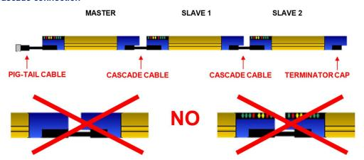
The Cascade connection can be done by using two or three Light Curtains (Standard Model), which can have different length and resolution.
