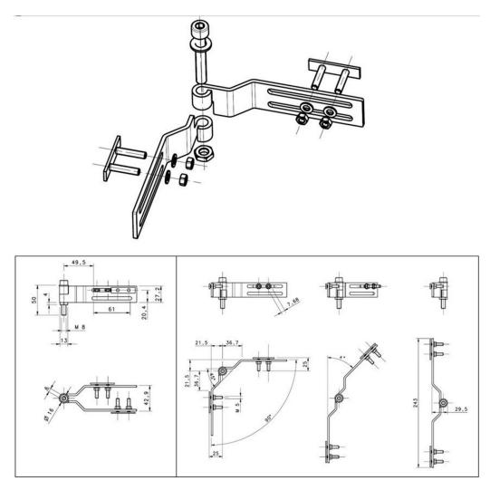
Figure 11 - Dimensions (mm)
