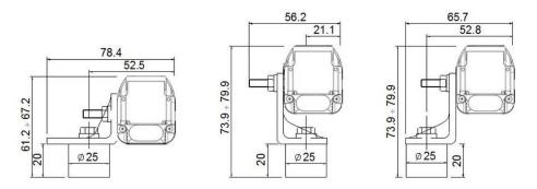
Figure 9 - Angled fixing bracket + Anti-vibration support
