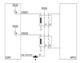
Figure 8 - EDM connection with manual restart selected on SG4-N models
