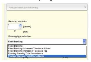
Figure 50 - ACM Configuration: Blanking configuration
