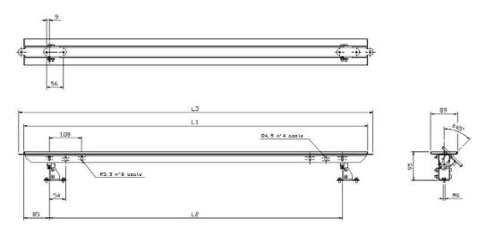
Figure 17 - Deviating mirrors (mm)
