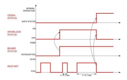
Figure 3 - SG4-N Restart timings (manual)
