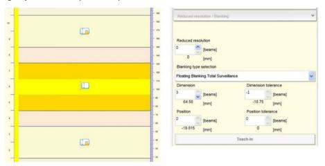
Figure 60 - Floating Blanking with total surveillance
