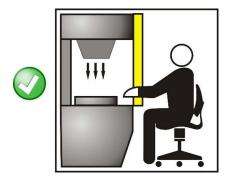
Figure 2 - Correct light curtain positioning
