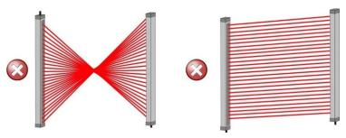
Figure 10 - Wrong light curtain TX-RX orientations
