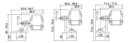
Figure 10 - Angled fixing bracket + Orientable support + Anti-vibration support
