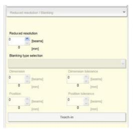
Figure 49 - ACM Configuration: Teach-in operation
