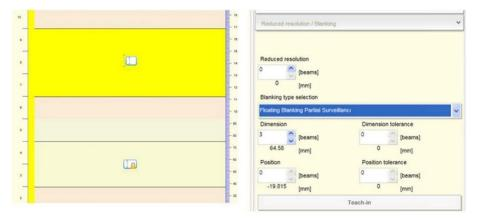
Figure 61 - Floating blanking with partial surveillance
