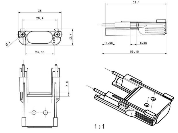
Fig 77 - Dimensions (mm)
