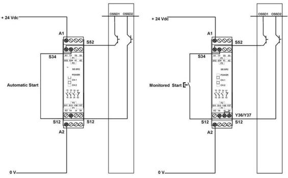
Fig 31 - Connection to SE-SR2 Safety Relais
