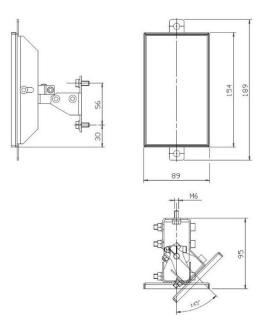
Fig 95 - SG-DM 150 Dimensions (mm)
