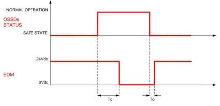
Fig 49 - EDM timings (PNP configuration)
