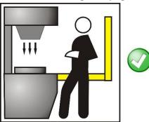
Fig 12 - Correct light curtain positioning
