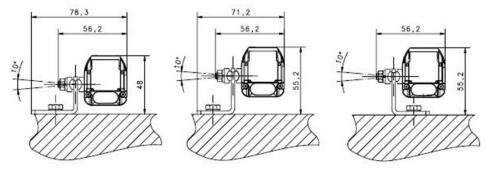
Fig 81 - Angled fixing bracket + Orientable support
