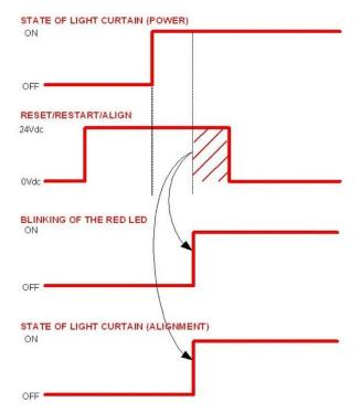
Fig 35 - Alignment timings
