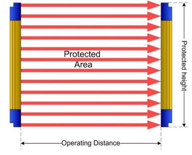
The controlled height is the height protected by the safety light curtain.
