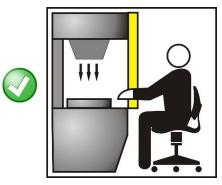
Fig 10 - Correct light curtain positioning
