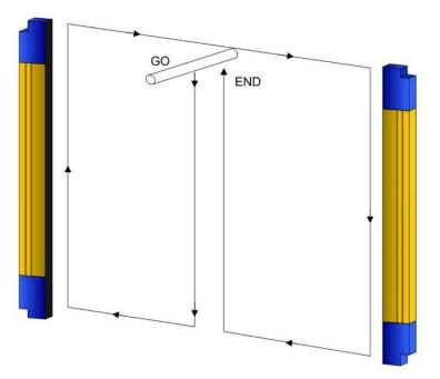
Fig 20 - Path of the test piece
