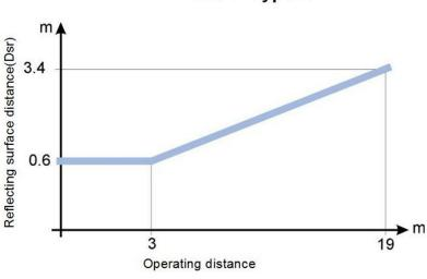
Fig 14 - Minimum distance from reflective surface
