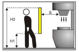
Fig 4 - Installation distance (vertical positioning)
