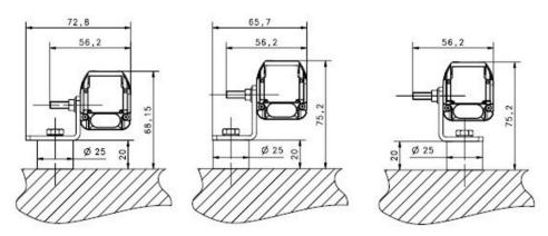
Fig 82 - Angled fixing bracket + Antivibration support
