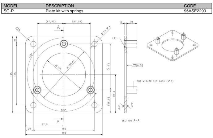
Fig 91 - Dimensions (mm)
