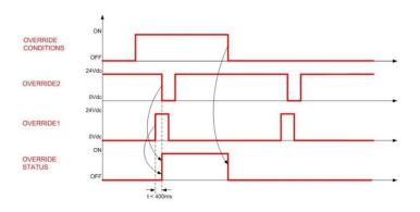
Fig 69 - Override timings (edge trigger)
