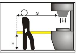
Fig 5 - Installation distance (horizontal positioning)
