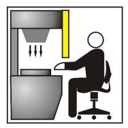
Fig 9 - Wrong light curtain positioning
