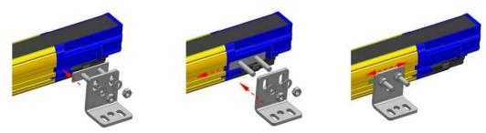
Fig 21 - Fixed brackets mounting procedure
