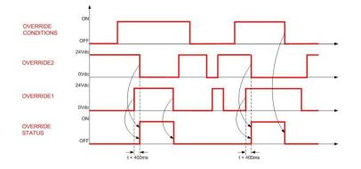
Fig 68 - Override timings (level trigger)
