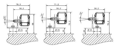
Fig 83 - Angled fixing bracket + Orientable support + Antivibration support
