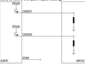
Fig 50 - EDM connection (PNP configuration)
