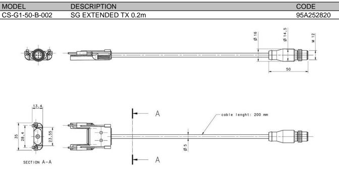
Fig 98 - TX - Pigtail cable
