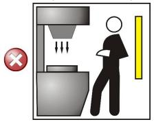
Fig 11 - Wrong light curtain positioning
