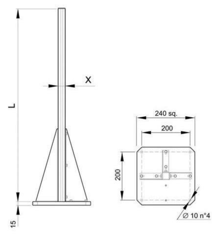
Fig 93 - Dimensions (mm)
