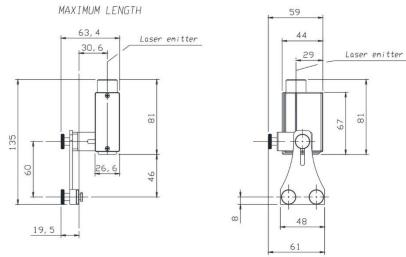
Fig 100 - Dimensions (mm)
