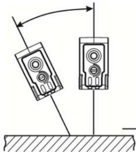
In the presence of moving backgrounds like conveyor belts, especially having a dark or shiny surface, the best object detection performance can be obtained by mounting the sensor at an angle (max 30°) with respect to the horizontal plane, as shown in the figure.
