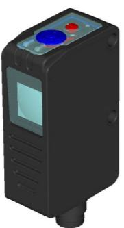
The operating distance is measured from the front surface of the sensor optics. Mark detection on a reflective surface is improved adjusting the beam direction to 5° ... 20° from surface axis.
