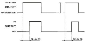
To set the DELAY ON function select in the menu parameters the "dlOn" text. d IUn
