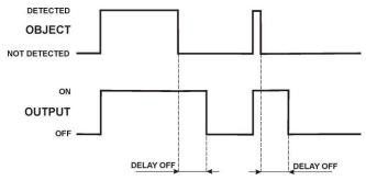
To set the DELAY OFF function select the "dIOF" text from the parameter menu
