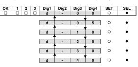
At each pressure of the SEL pushbutton, the different delay levels in ms are visualised in a cvclical manner at the output deactivation and moreover, the relative delay value will be stored. When the "d-00" message is visualised the operating mode will be "run", and "rund" in all other cases.
