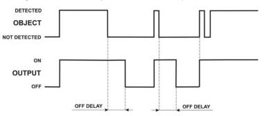
The delay adjustment is carried-out manually using the Timer adjustment trimmer. Clockwise rotation increase the delay from 0 to a max. 1 sec. value.
