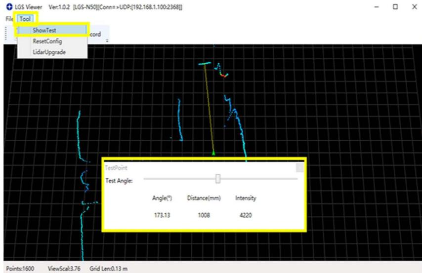
Angles start from  $0^{\circ}$  in the point behind the LiDAR and go on clockwise up to  $360^{\circ}$ :
