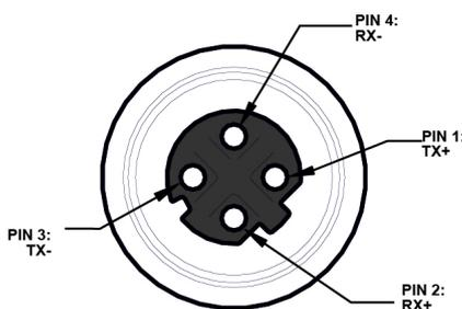
Figure 6 - Ethernet connector
