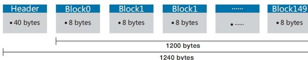
**Figure 12 - Format of point cloud information packet**
