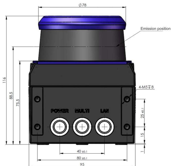
Figure 2 - LGS-N50 Back Mounting interface
