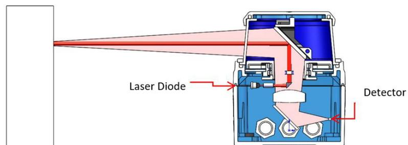
**Figure 1 - LGS-N50 LiDAR working principle**
