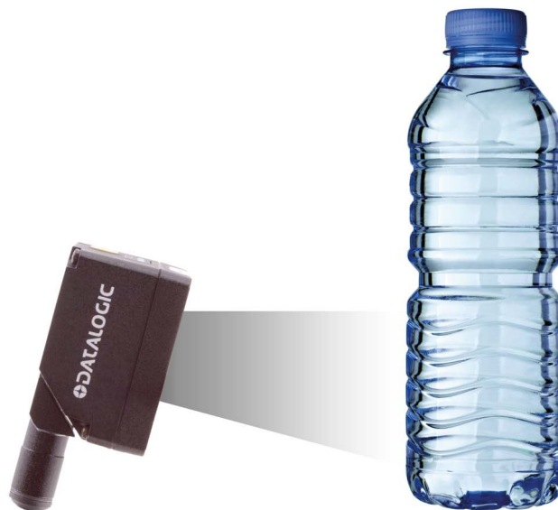
Figure 5 - Max. 20% pitch to avoid direct reflections
