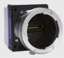
Line scan cameras use the GigE Vision standard. These cameras are for applications that need high resolution and the object is very long or an endless web of material. The cameras are the ideal solution for printing machines to inspect printed images such as a continuous web or the printing around a circular object.
