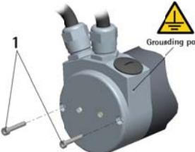
1 Connect the cable shield to cable gland.
