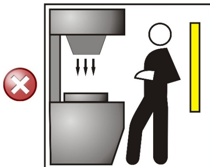
Fig 11 - Wrong light curtain positioning
