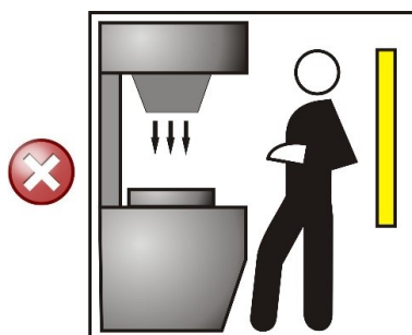
Figure 7: Wrong light curtain positioning
