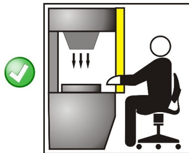
Figure 6: Correct light curtain positioning
