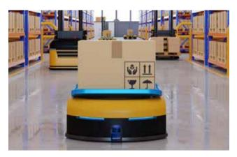
With an operating temperature range of -20 ...+50 °C, an IP66 protection against dust and water, and its sturdy compact structure, Lidar Guidance Scanner is well suited for use in indoor industrial environments.
