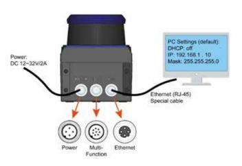
The configuration of Lidar Guidance Scanner parameters doesn't require any special software: an integrated web server allows to visualize and change parameters with any browser.
